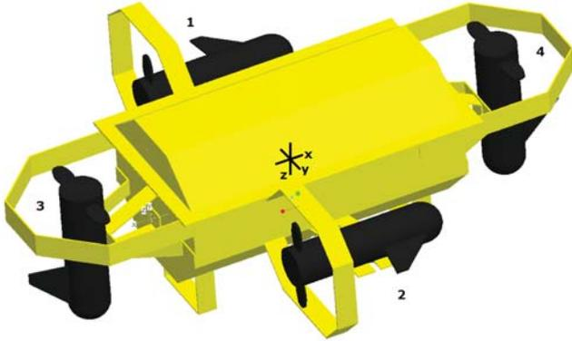
Fig. 4. Three dimensional CAD made for PoseiBoT. Notice the location, translation direction and thrusters enumeration.
