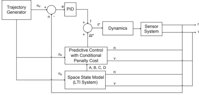
Fig. 3. Predictive control scheme implemented in this application. The main subsystems required for this application were: trajectory generator, model linearizer and predictive controller.
