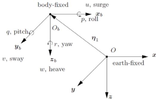
Fig. 2. Body and earth fixed reference frames [16].
