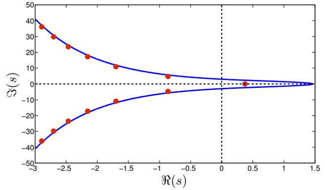
Fig. 1. Envelop and zeros of  $\Delta(s) = s + 1 - 2e^{-s}$
