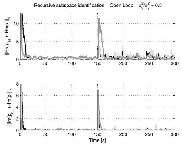
Fig. 2. Real and imaginary part of the estimated eigenvalues - open loop experiment -  $\frac{\sigma_v^2}{\sigma_y^2} = 0.5$ .
