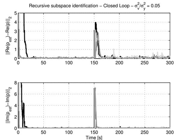
Fig. 3. Real and imaginary part of the estimated eigenvalues - closed loop experiment -  $\frac{\sigma_v^2}{\sigma_y^2} = 0.05$ .
