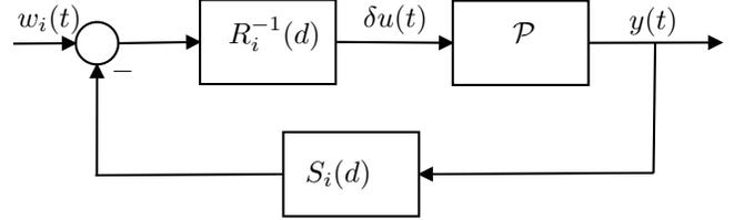
Fig. 4. Potential loop associated to definition of  $w_i$ .
