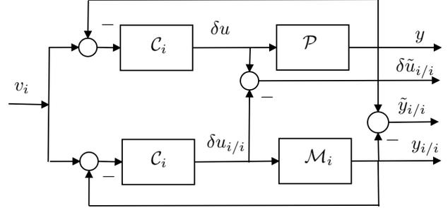
Fig. 2. Detail of a multiple-model switching control.
