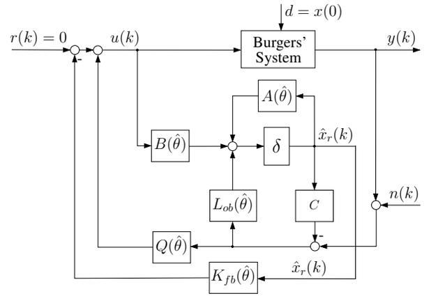
Fig. 3. Block diagram of the observer-based LPV controller
