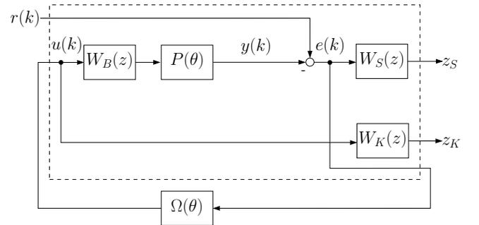
Fig. 2. Generalized plant for the synthesis of output feedback LPV controller
