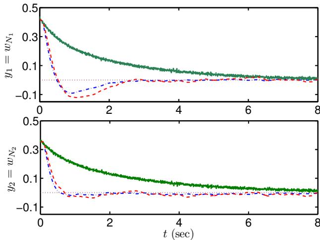
Fig. 4. Rejection of a non-zero initial condition disturbance by observer-based state feedback LPV (dashed), output feedback LPV with a nonlinear observer (dashed-dotted) and LQG (solid) controllers
