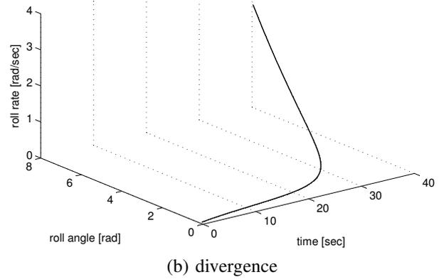
Fig. 3. Uncontrolled wing rock dynamics
