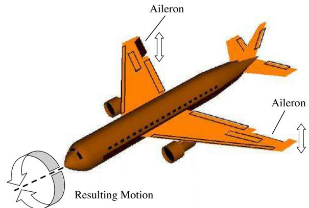
Fig. 1. Aileron deflection influence on the roll motion, modified from <http://en.wikipedia.org/wiki/Aileron>
