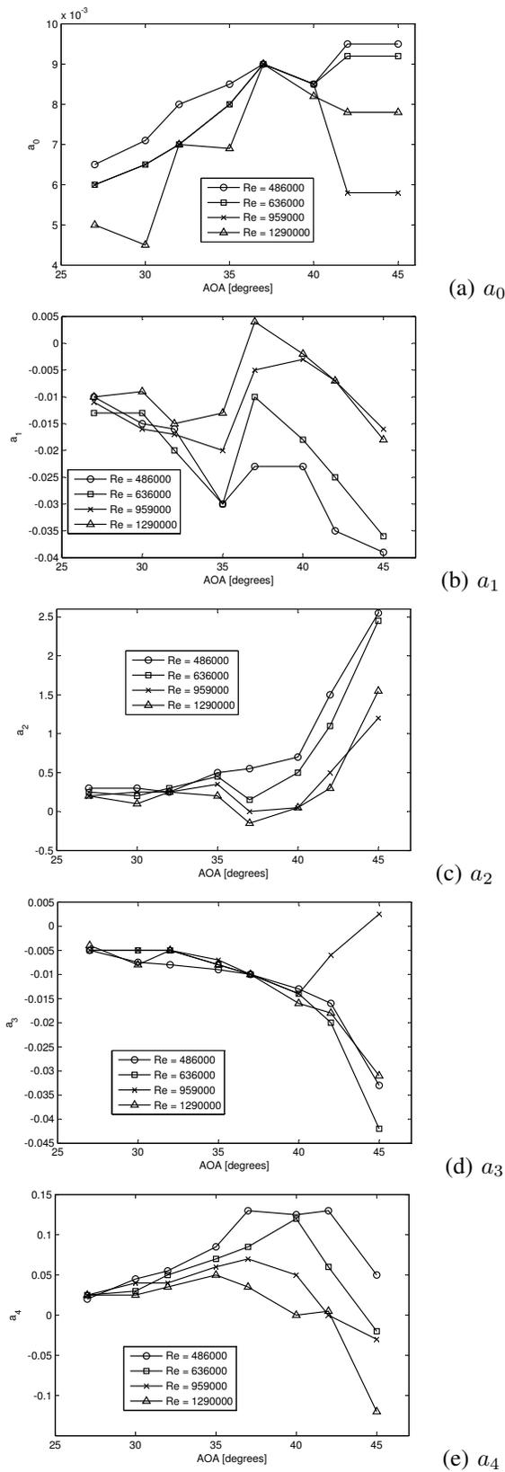
Fig. 2. The coefficients  $a_0, \dots, a_4$  corresponding to different AOA and Reynolds number  $Re$  from [2]
