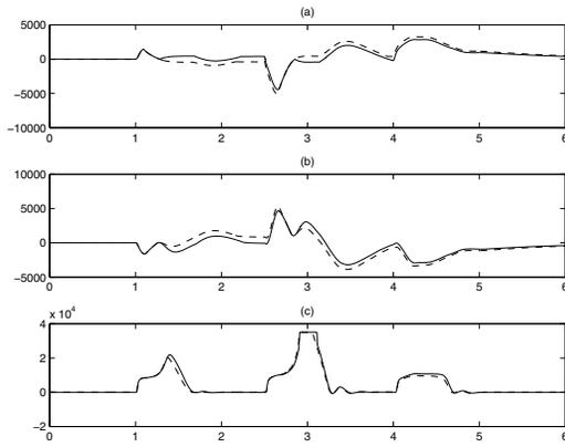
Fig. 3. (a)  $F_{y,f}$  with limiting function (solid),  $F_{y,f}$  with linear saturation function (dashed) [N] vs time [s]; (b)  $M_z$  with limiting function (solid),  $M_z$  with linear saturation function (dashed) [Nm] vs time [s]; (c)  $b_x$  with limiting function (solid),  $b_x$  with linear saturation function (dashed) [Nm rad/s] vs time [s]
