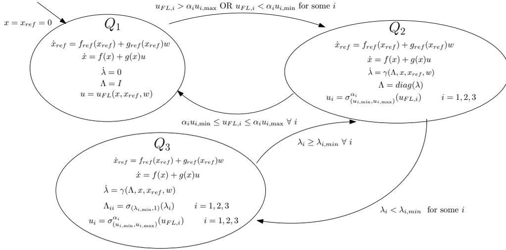
Fig. 1. Hybrid Model of vehicle controlled with linearizing feedback, limiting functions and reference modification. In the first state, the nominal reference is tracked exponentially. In the second state, at least one of the actuators is getting to saturation, so the reference is modified accordingly and the linearizing feedback is limited. In the third case, the reference modification reaches its limiting point for at least one of the state variables.
