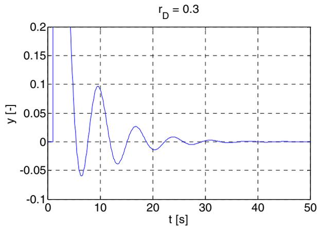
Fig. 5. Disturbance response course when  $r_D = 0.3$  (the first peak of size 0.35 is not shown in full size in the figure).
