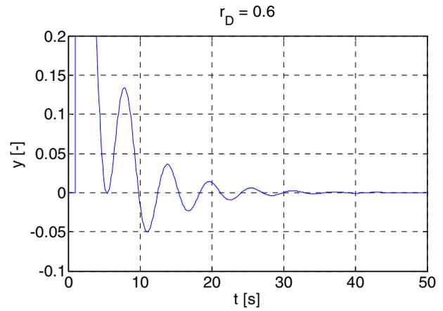
Fig. 8. Disturbance response course when  $r_D = 0.6$  (the first peak of size 0.35 is not shown in full size in the figure).
