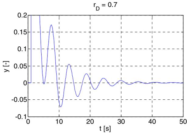
Fig. 10. Disturbance response course when  $r_D = 0.7$  (the first peak of size 0.35 is not shown in full size in the figure).
