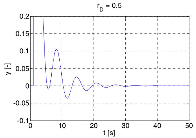
Fig. 7. Disturbance response course when  $r_D = 0.5$  (the first peak of size 0.35 is not shown in full size in the figure).
