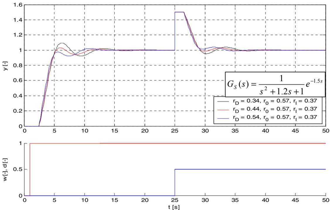
Fig. 12. Example of control process using the controller with setting obtained with the presented derivative component tuning rule (slightly better courses with higher  $r_D$  values than the found one are shown for comparison)
