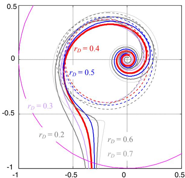
Fig. 3. Nyquist plots for PID controller with various  $r_D$  setting
