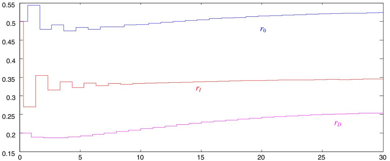
Fig. 9. Example of PID controller tuning  $\left( G_{PID} = r_0 + \frac{r_I}{s} + r_D s \right)$ .
