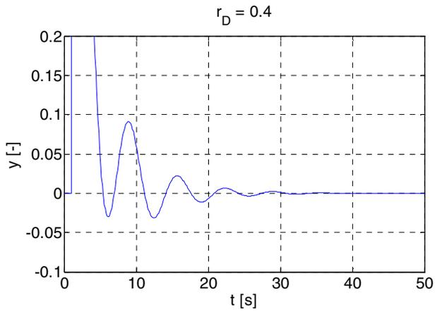
Fig. 6. Disturbance response course when  $r_D = 0.4$  (the first peak of size 0.35 is not shown in full size in the figure).
