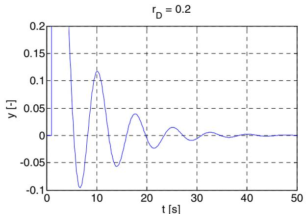
Fig. 4. Disturbance response course when  $r_D = 0.2$  (the first peak of size 0.35 is not shown in full size in the figure as it has no illustrative value, it occurs always in the same size due the presence of time delay).
