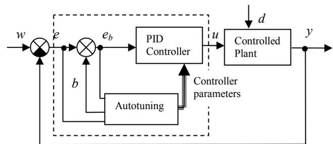
Fig. 1. Scheme of a control circuit with an added autotuning mechanism.
