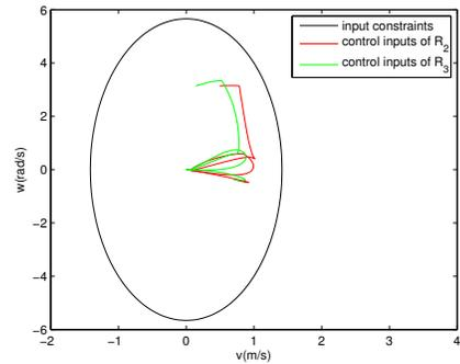
Fig. 8: Elliptic input constraints and control inputs of  $R_2$  and  $R_3$ .
