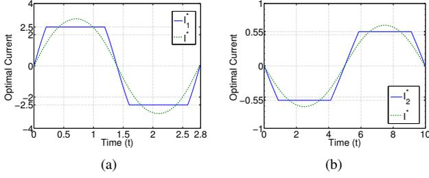
Fig. 4. Optimal bounded and unbounded controls for the sinusoidal PRC with parameters  $z_d = 1$  and  $\omega = 1$  (a) for  $T = 2.8$  with the bound  $M = 2.5$  and (b) for  $T = 10$  with the bound  $M = 0.55$ .
