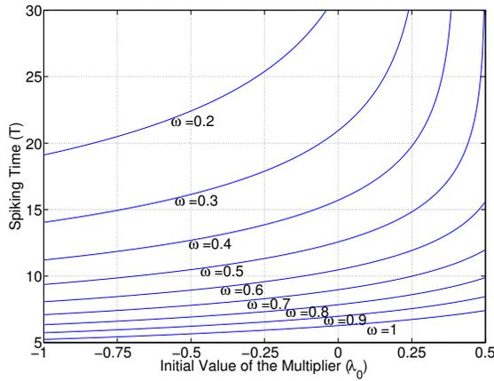
Fig. 2. Variation of the spiking time,  $T$ , with the initial multiplier,  $\lambda_0$ , for different  $\omega$  values and  $z_d = 1$ .
