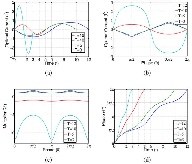
Fig. 3. (a) Variation of the minimum-power control,  $I^*$ , with time,  $t$ . (b) Variation of  $I^*$  with phase  $\theta$ . (c) Variation of the optimal multiplier,  $\lambda^*$ , with  $\theta$ . (d) Variation of the phase,  $\theta^*$ , with  $t$ , for the sinusoidal PRC with  $z_d = 1$  and  $\omega = 1$  for the spiking times,  $T = 3, 5, 10$  and  $12$ .
