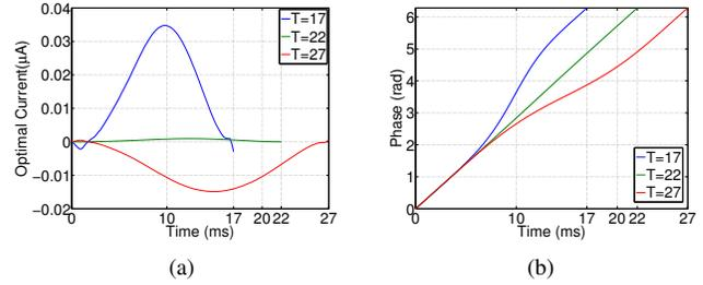
Fig. 7. (a) Optimal currents for various spiking times  $T = 17, 22, 27$  ms for the Morris-Lecar PRC. (b) The corresponding phase trajectories.
