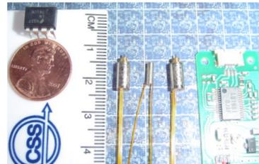
Figure 1. Mini-motors with ASICs: Actuators are fabricated utilizing *bulk* and surface micromachining technologies [7]
