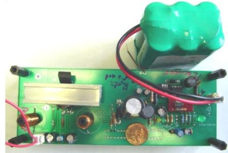
Figure 3. Electronic module of a high power density generation system
