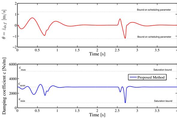
Fig. 3. Scheduling parameter and saturation constraint.
