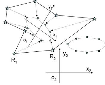
Fig. 3. step 3: robot  $R_1$  performs a rotation to find the best orientation of the TGP, and at the best location and orientation, it returns with the destinations for every robot.
