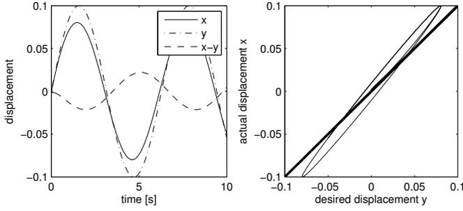
Fig. 1. Profile of trajectories with hysteresis for a sinusoidal reference  $y(t) = 0.1 \sin(t)$ . When the hysteresis disappears, the hysteretic loop in the right graph reduces to the bold straight line.
