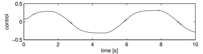
Fig. 3. Profile of control input for a sinusoidal reference.
