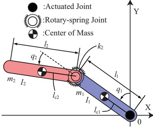
Fig. 1. AF robot: two-link flexible robot with a spring between two-links.
