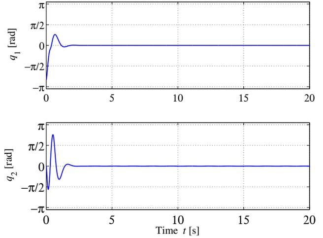
Fig. 5. Time responses of  $q_1$  and  $q_2$  under the swing-up control:  $k_2 = 1.5$ .
