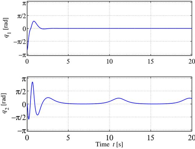
Fig. 3. Time responses of  $q_1$  and  $q_2$  of the swing-up control:  $k_2 = 1.0$ .
