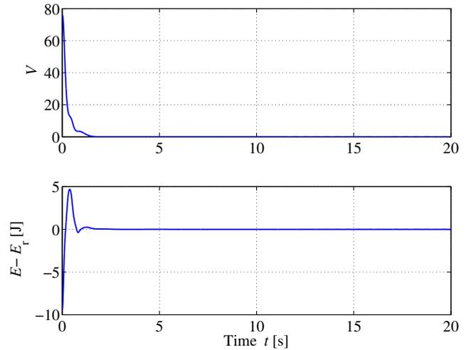
Fig. 2. Time responses of  $V$  and  $E - E_r$  of the swing-up control:  $k_2 = 1.0$ .
