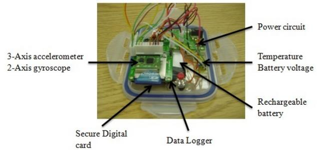
Fig. 2. Embedded device.
