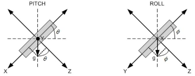
Fig. 5. Gravity components when wheelchair is tilted.
