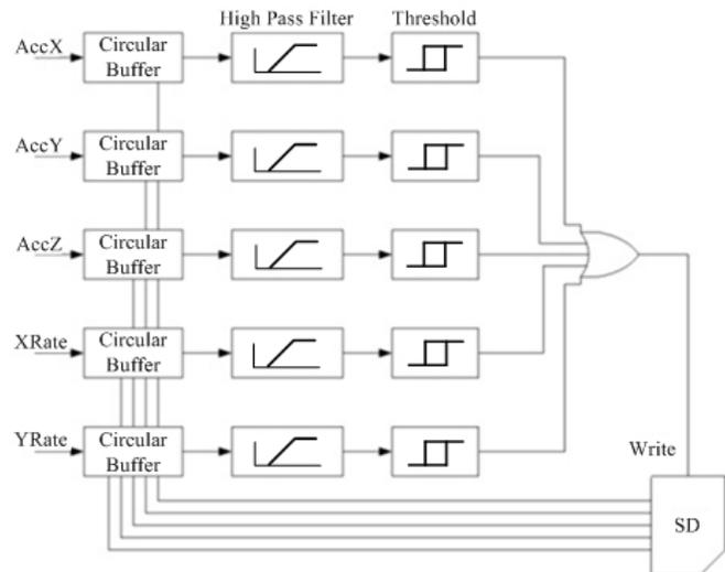
Fig. 3. Real-time signal processing algorithm for selective data storage.
