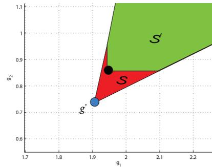
Fig. 6. Zoom on the no viable point  $g'$ : the point  $g'$  (blue) is not inside  $S'$ , having been substituted by a new viable vertex (black spot).
