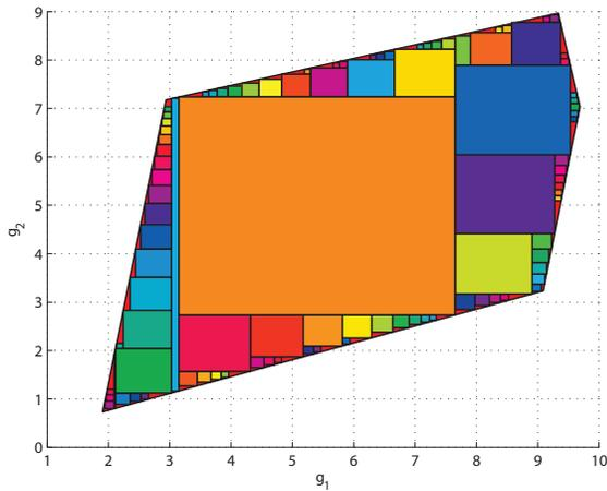
Fig. 4. Multi-inner box approximation  $\mathcal{M}(S) = \{\Omega_k\}_{k=1}^{91}$  of  $S$ .
