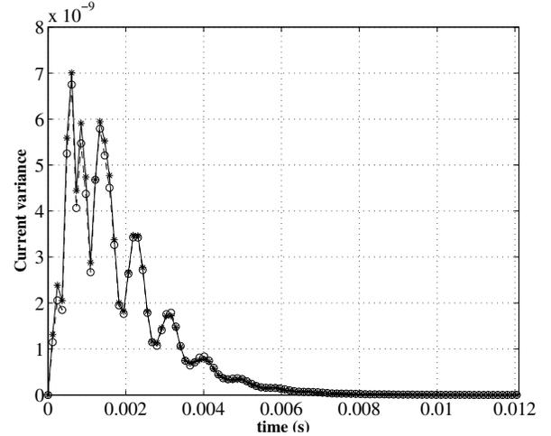
Fig. 2. Simulation example. Variances at  $t = t_i, i = 0, \dots, 99$  of the current  $i_L(t)$ , obtained either with MC simulations of the model (dashed line with 'o') or on the basis of the coefficients of the PCEs  $\hat{v}_1^*(t_i, \boldsymbol{\kappa})$  (solid line with '\*').
