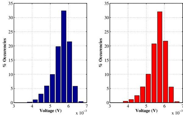
Fig. 3. Simulation example. Comparison between the p.d.f. of variable  $v_C(t_{21}, \kappa)$  either with 27000 MC simulation with the system model (left) or with 27000 MC evaluations of the PCE  $\hat{v}_2^*(t_{21}, \kappa)$  (right).
