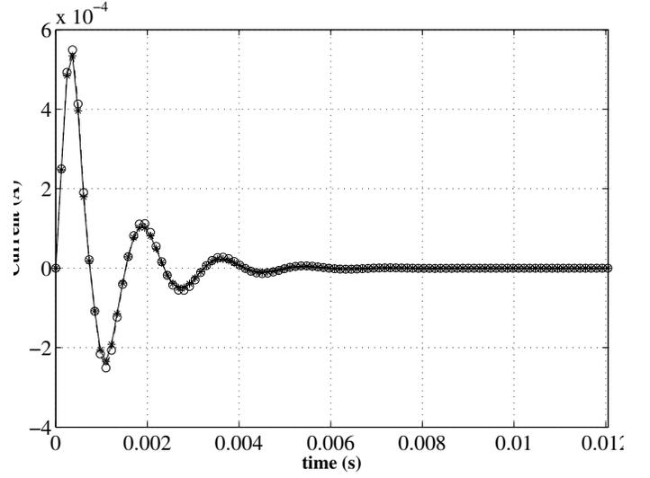
Fig. 1. Simulation example. Mean values at  $t = t_i, i = 0, \dots, 99$  of the current  $i_L(t)$ , obtained either with MC simulations of the model (dashed line with 'o') or with the coefficients of the term of degree 0 in their respective PCEs  $\hat{v}_1^*(t_i, \boldsymbol{\kappa})$  (solid line with '\*').
