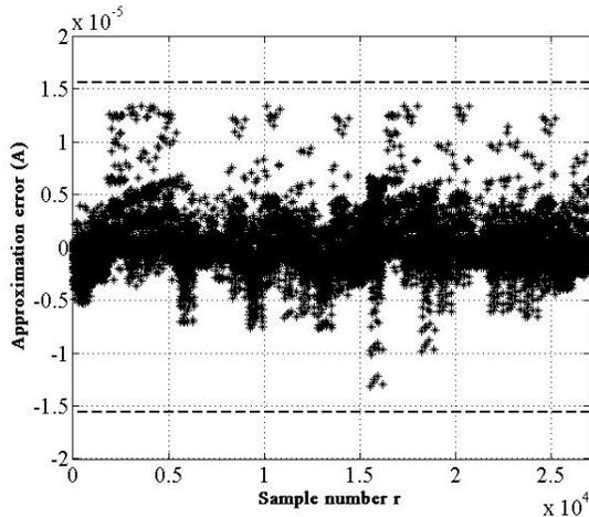
Fig. 4. Simulation example. Approximation errors  $\Delta_1^*(t_9, \kappa)$  (\*) and worst-case bounds  $\pm\zeta_{2,9}$  (dashed lines).
