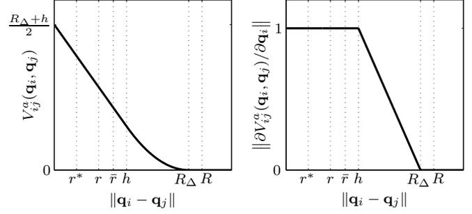
Fig. 2. Bounded avoidance function and bounded avoidance control.
