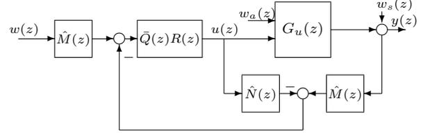
Fig. 5. An equivalent form of the data-driven realization of the EIMC structure
