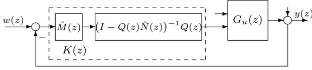
Fig. 2. An equivalent realization of the Youla parameterization
