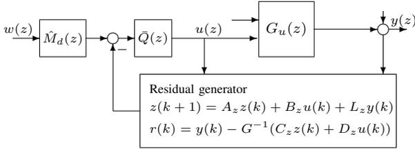
Fig. 4. A data-driven realization of the EIMC structure
