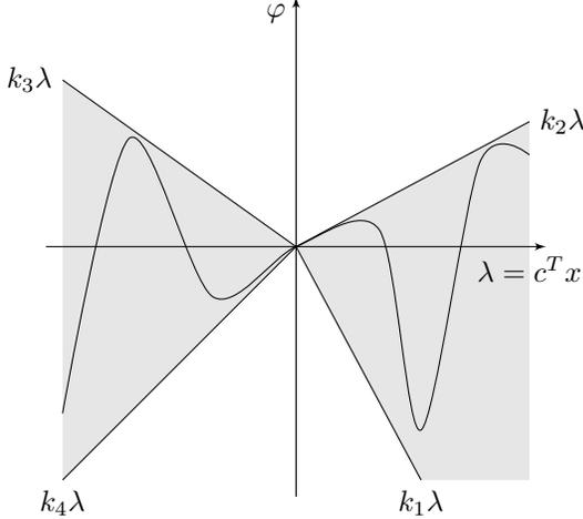
Fig. 3. Asymmetric domain of the feedback characteristic.
