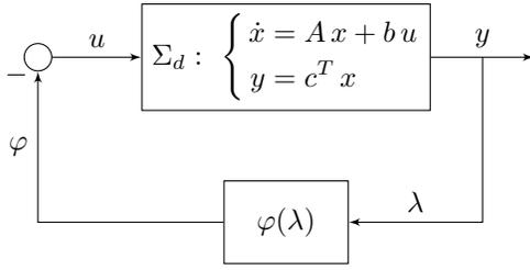
Fig. 2. Block diagram of the Lur'e system.
