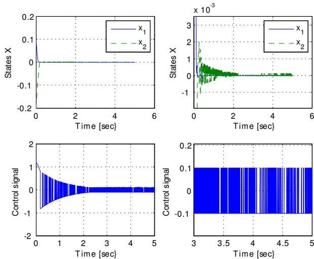
Fig. 3. The states and the control signal (with the zoom) for the super-twist controller with adaptation of the gain parameter  $\beta$  based on the "equivalent control" signal.
