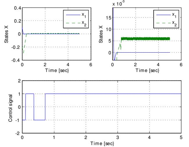
Fig. 1. The states and the control signal for the super-twist controller without adaptation of the gain parameter  $\beta$ .
