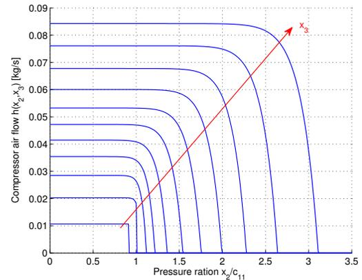
Fig. 1. Compressor map: the curves are parameterized by  $x_3$ , and grow when it increases
