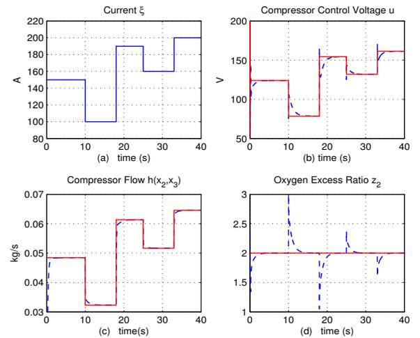
Fig. 2. Simulation response of the closed-loop system with the PI controller
