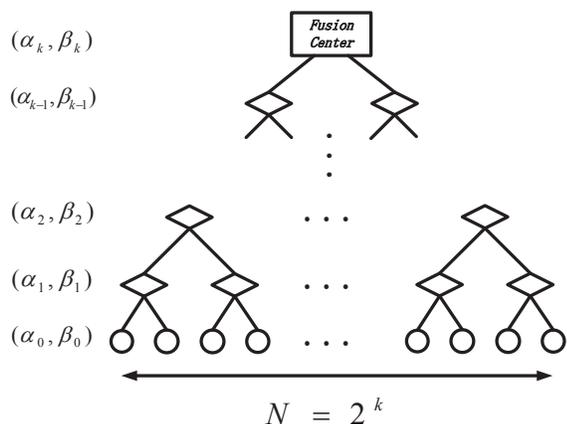
Fig. 1. A balanced binary relay tree with height  $k$ . Circles represent sensors making measurements. Diamonds represent relay nodes which fuse binary messages. The rectangle at the root represents the fusion center making an overall decision.
