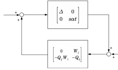
Fig. 3. IMC anti-windup expressed in the standard feedback connection.
