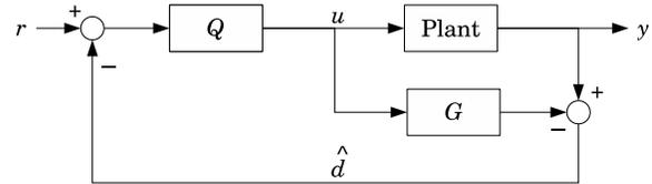
Fig. 1. Conventional IMC structure.
