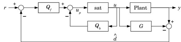
Fig. 2. IMC anti-windup structure.
