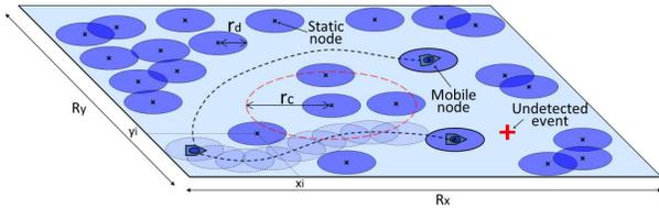
Fig. 1. Mixed sensor network model.
