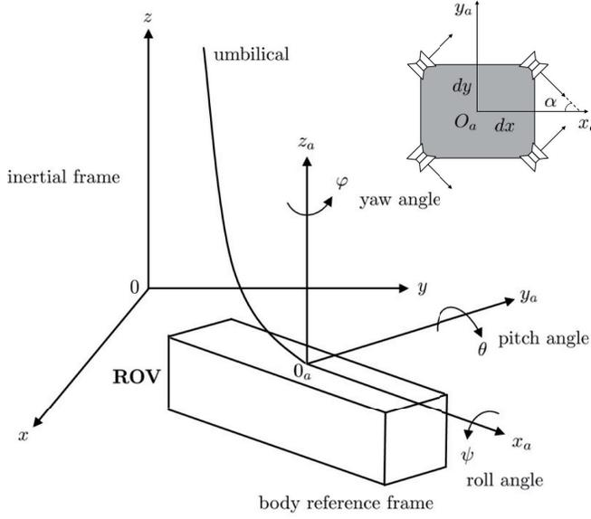
Fig. 1. ROV operational configuration.
