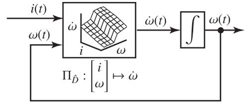
Fig. 7: Data-based PWA model for DC motor system
