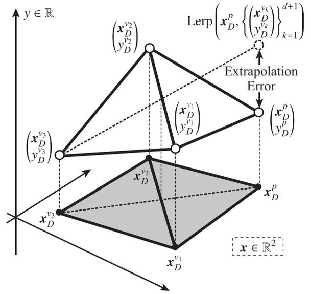
Fig. 5: Illustration of extrapolation error ( $d = 2$ )
