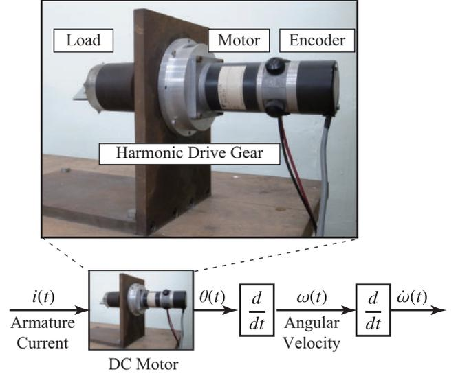
Fig. 6: DC motor system
