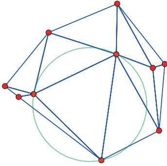
Fig. 3: An example of Delaunay triangulation for set  $P$  of points in the plane. No point in  $P$  is inside the circumcircle of any triangle.
