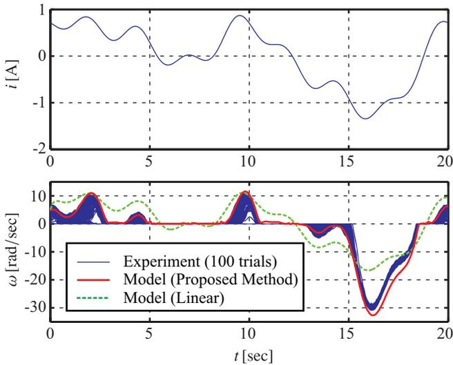
Fig. 9: Validation input and output of the experiment system and the model obtained with moderate compression level ( $w = 5 \times 10^{-3}$ )
