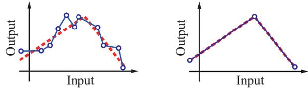
(a) Data-based PWA model directly built from measured data, which fluctuated by stochastic noise. (b) Ideal data-based PWA model for the example system.
