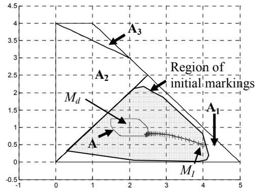
Figure 3: Control design in finite time in a single region: marking trajectory in plan  $(m_1, m_2)$  to drive  $M(t, M_l)$  from  $M_l$  to  $M_d$  in  $\mathbf{A}_1$ .
