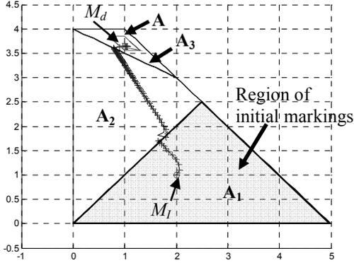
Figure 4: Control design in finite time with sequence  $S = A_1, A_2, A_3$ : marking trajectory in plan  $(m_1, m_2)$  to drive  $M(t, M_i)$  from  $M_1$  to  $M_d$  in  $A_3$ .
