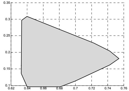
Figure 2: Control design in finite time in a single region: region of CBIC control actions in plan  $(u_1, u_2)$  to drive  $M(t, M_l)$  from  $M_l$  to  $M_d$  in  $\mathbf{A}_1$ .
