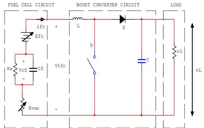
Fig. 3 Circuit Diagram of Fuel Cell and DC-DC converter
