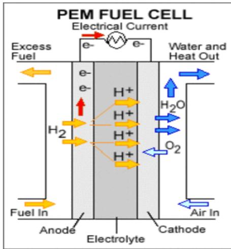
Fig. 1 Schematic of a Fuel cell
