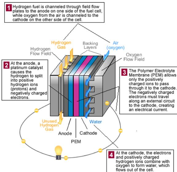
Fig. 2 Detailed Schematic of the PEMFC operation
