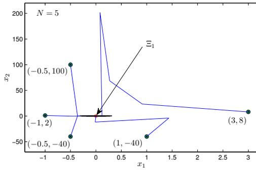
Fig. 2. Sample closed-loop trajectories under the RMNT control in nominal conditions
