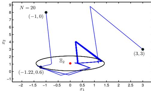
Fig. 3. Sample closed-loop trajectories under the RMNT control in nominal conditions, with a non robustly controllable target set  $\Xi_2$ . From the initial point  $x_0 = (-1.22, 0.6) \in \Xi_2$  the state cannot be kept inside  $\Xi_2$  with the available control input. The trajectories asymptotically reach a triangle-shaped limit-cycle condition which temporarily leaves the target set
