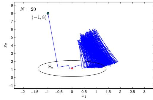
Fig. 4. Sample closed-loop trajectory under the RMNT control with bounded perturbations. The trajectory remains bounded in perturbed conditions despite a non robust positively controllable target set has been used
