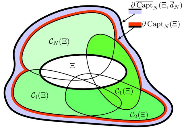
Fig. 1. Scheme of the sets involved in the statement and proof of Theorem 2.1.  $\text{Capt}_N(\Xi)$  denotes the  $N$ -steps capture basin of  $\Xi$ , while  $\overline{\text{Capt}}_N(\Xi, \bar{d}_N)$  is an extension of the nominal capture basin (see (10)) that can be proven to be robust positively controllable. That is, there exists a control law, compliant with the input constraints, that renders  $\overline{\text{Capt}}_N(\Xi, \bar{d}_N)$  RPI.
