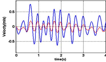
Fig. (8-b). Velocity tracking, utilizing Conventional Three Channel architecture. When time < 4 sec
