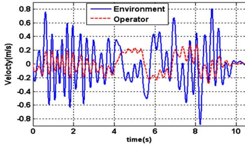
Fig. (8-a). Velocity tracking, conventional Three Channel architecture.
