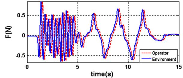
Fig. (11). Force tracking, utilizing PTC, communication delay=140 ms.
