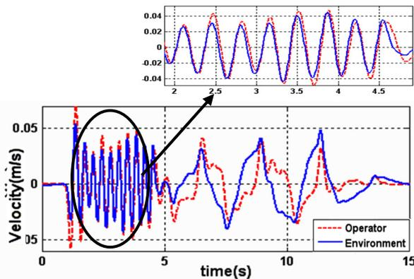
Fig. (10). Velocity tracking, for PTC, communication delay=140 ms
