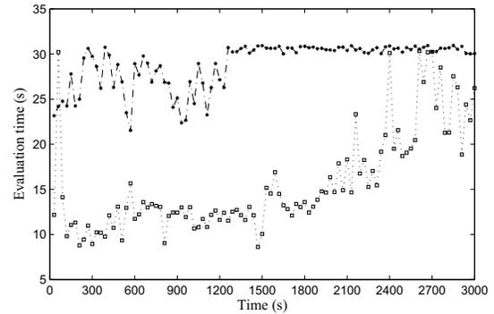
Fig. 5. The total evaluation time needed for each evaluation of each MPC method. Centralized LMPC (solid line with \*), iterative DMPC with one evaluation (dotted line with  $\square$ ). The prediction horizon  $N = 5$ .
