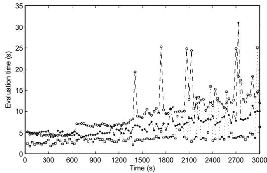
Fig. 4. The total evaluation time needed for each evaluation of each MPC method. Centralized LMPC (solid line with \*), sequential DMPC (dashed line with  $\circ$ ), and iterative DMPC with one evaluation (dotted line with  $\square$ ). The prediction horizon  $N = 2$ .
