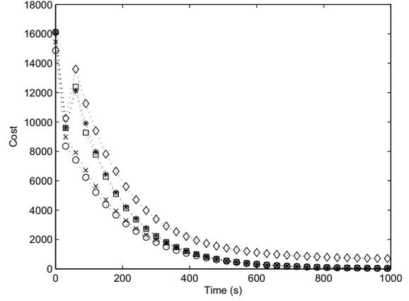
Fig. 2. The costs of the closed-loop system under the centralized LMPC ( $\circ$ ), the sequential DMPC ( $*$ ), and the iterative DMPC with one evaluation ( $\square$ ) and with two evaluations ( $\times$ ), and the iterative DMPC with one evaluation ( $\diamond$ ) under uncertainty. The prediction horizon  $N = 1$ .
