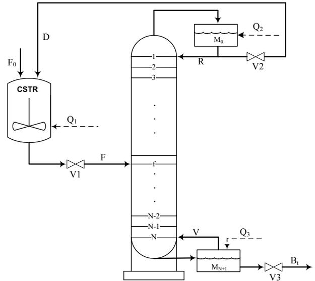
Fig. 1. Process schematic.
