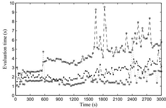
Fig. 3. The total evaluation time needed for each evaluation of each MPC method. Centralized LMPC (solid line with \*), sequential DMPC (dashed line with  $\circ$ ), and iterative DMPC with one evaluation (dotted line with  $\square$ ). The prediction horizon  $N = 1$ .
