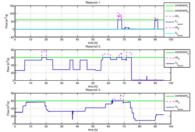
Fig. 3. Turbine flows (Control inputs  $\mathbf{u}_i^{opt}$  and references  $\mathbf{u}_{s_i}$ ).
