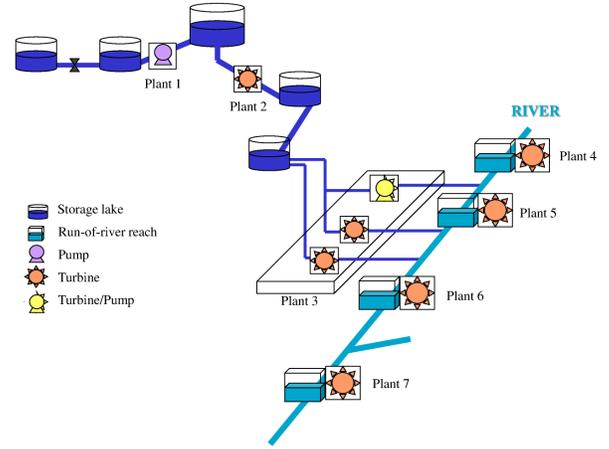
Fig. 1. The Hydro-power valley configuration.
