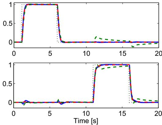
Fig. 4. Comparison between existing iterative methods and VRFT for LV100 control design in a noise-free context. Reference signals (dotted) and achieved responses: with IFT controller (light dashed), with CbT controller (dash-dot) and with MIMO VRFT controller (solid). The desired response is also shown (dark dashed) but it is almost completely overlapped with CbT.
