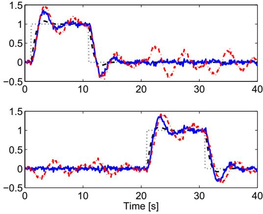
Fig. 3. Closed-loop responses to step reference excitation (dotted):  $M$  (dashed), closed-loop with VRFT SISO controller (dash-dot) and closed-loop with VRFT MIMO controller (solid).
