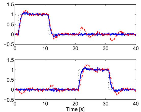
Fig. 2. Closed-loop responses to step reference excitation (dotted):  $M$  (dashed), closed-loop with VRFT SISO controller (dash-dot) and closed-loop with VRFT MIMO controller (solid). Notice that dashed and solid line are almost overlapped.
