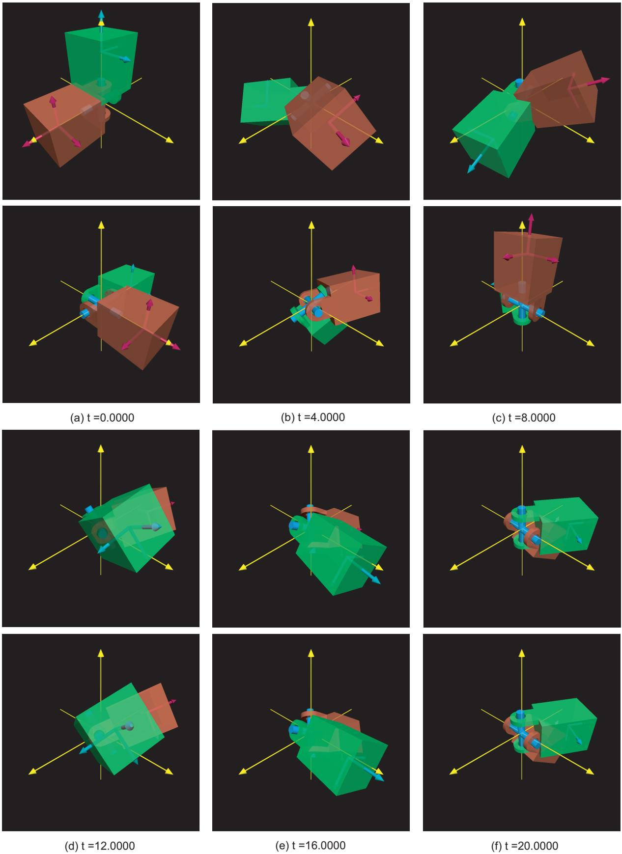
Fig. 5 Snapshot in Trajectory Tracking Control (Upper: Desired Trajectory, Lower: Result)
