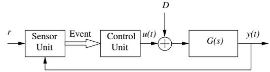
Fig. 1. Scheme of the event-based control system.
