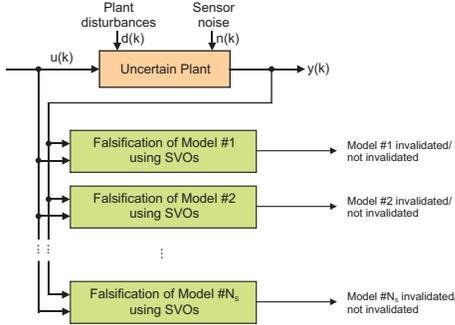
Fig. 4. Multiple-model falsification architecture using SVOs.
