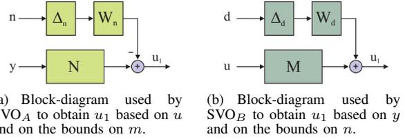
Fig. 2. Block-diagrams used to compute the set-valued estimates of  $u_1$ .
