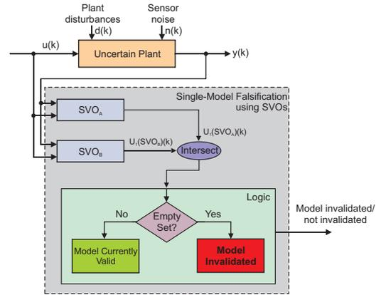
Fig. 3. Architecture for single-model falsification using SVOs, including the interconnection between the *true* plant,  $SVO_A$  and  $SVO_B$ .
