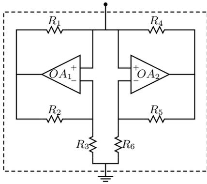
Fig. 2. Operational Amplifier realization of Chua's diode.
