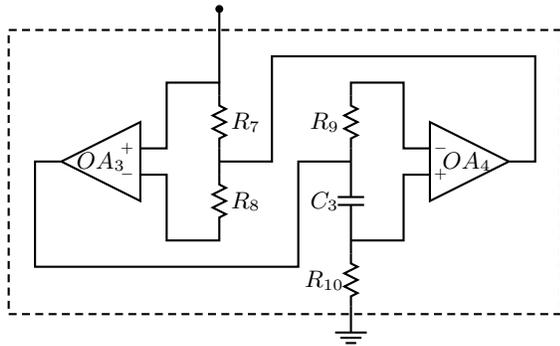
Fig. 3. Equivalent circuit for the inductor in Chua's circuit.
