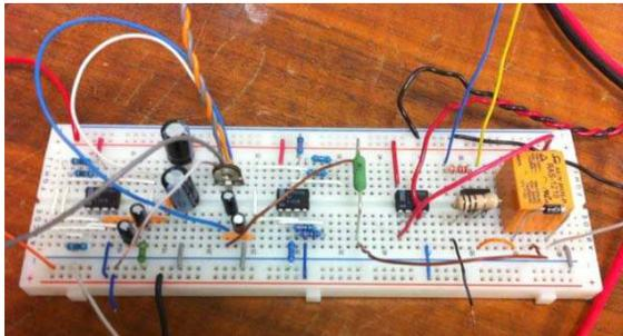
Fig. 4. Modified Chua's circuit prototype.
