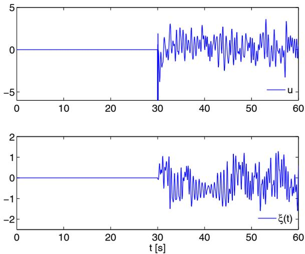
Fig. 7. Control input signal,  $u$ , and on-line GPI observer estimation,  $\hat{\xi}(t)$ , of the lumped disturbance input.
