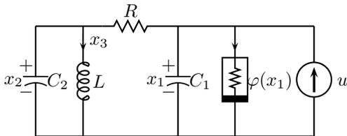
Fig. 1. Controlled Chua’s circuit
