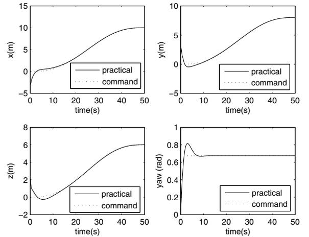
Fig. 1. The trajectory of the controlled autonomous helicopter
