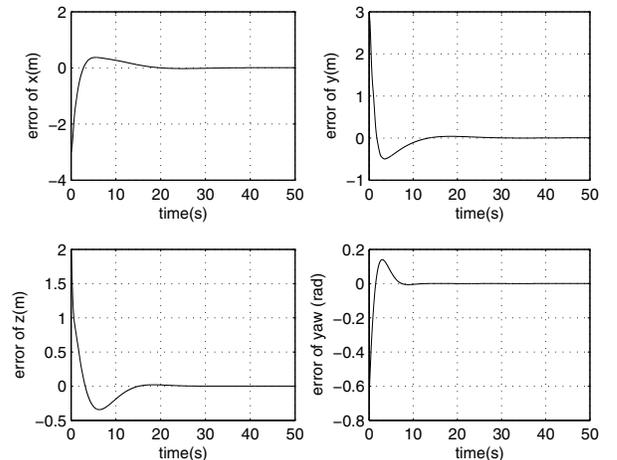
Fig. 2. The tracking errors of the controlled autonomous helicopter
