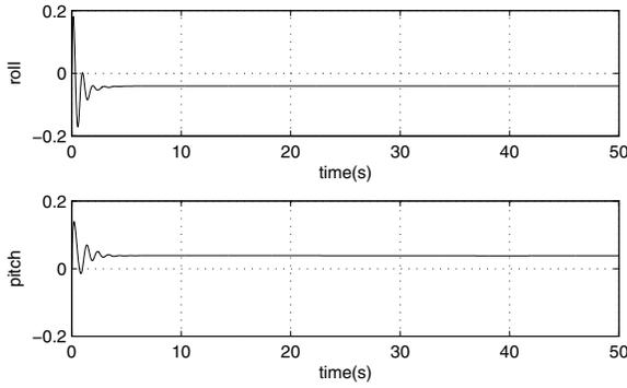
Fig. 3. The roll and pitch angle of the controlled autonomous helicopter
