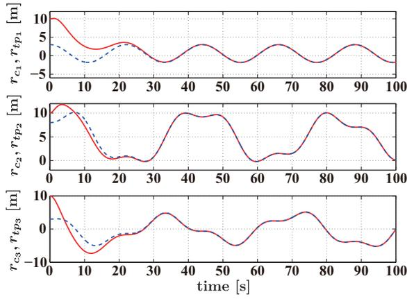
Fig. 2. PD controller: responses of position (left) and attitude (right) of chaser (solid line) and target (dashed line).
