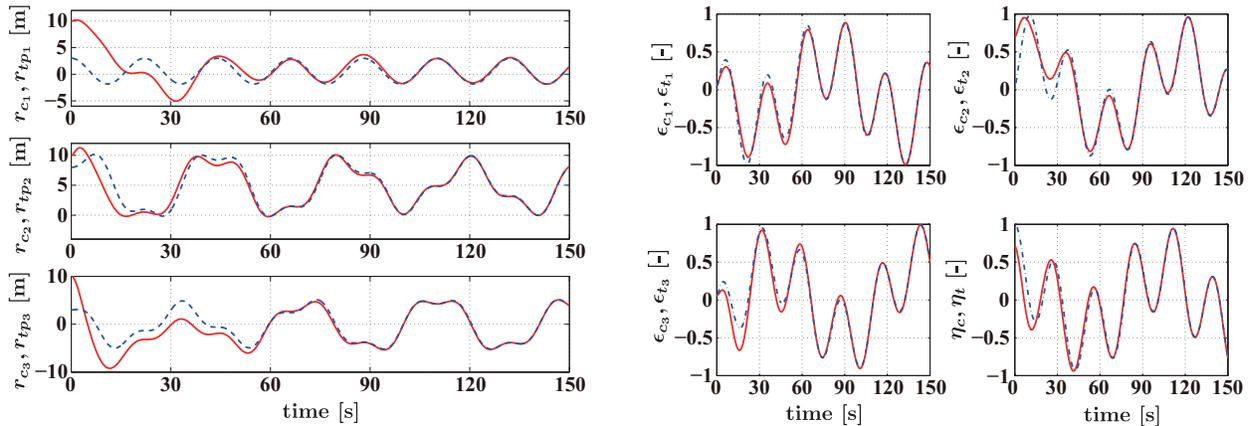
Fig. 6. PID controller (Case 3) : responses of position (left) and attitude (right) of chaser (solid line) and target (dashed line) under constant disturbance.
