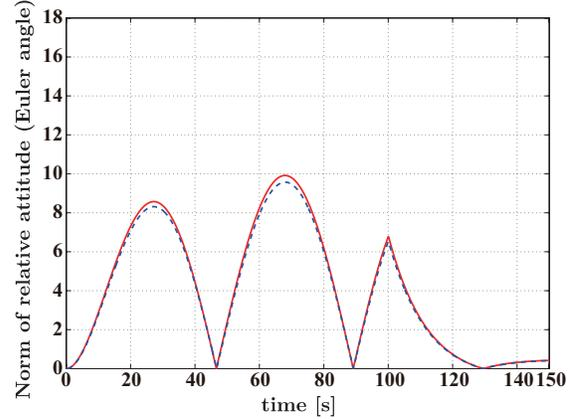
Fig. 8. PID  $\mathcal{H}_\infty$  controller: responses of norms of relative position (left) and attitude (right) for  $\gamma = 0.8$  (solid line) and  $\gamma = 0.4$  (dotted line).
