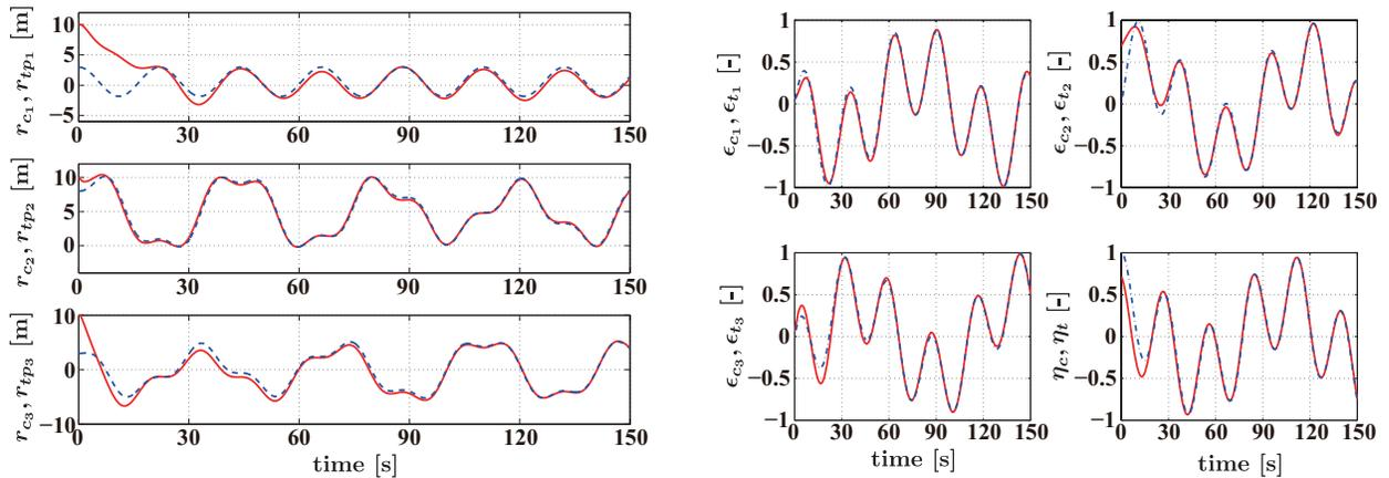
Fig. 5. PD  $\mathcal{H}_\infty$  controller (Case 2) : responses of position (left) and attitude (right) of chaser (solid line) and target (dashed line) under constant disturbance.
