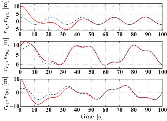
Fig. 3. PID controller: responses of position (left) and attitude (right) of chaser (solid line) and target (dashed line).
