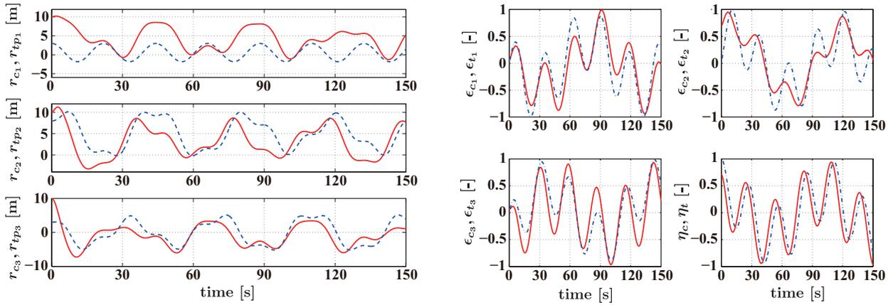
Fig. 4. PD controller (Case 1) : responses of position (left) and attitude (right) of chaser (solid line) and target (dashed line) under constant disturbance.
