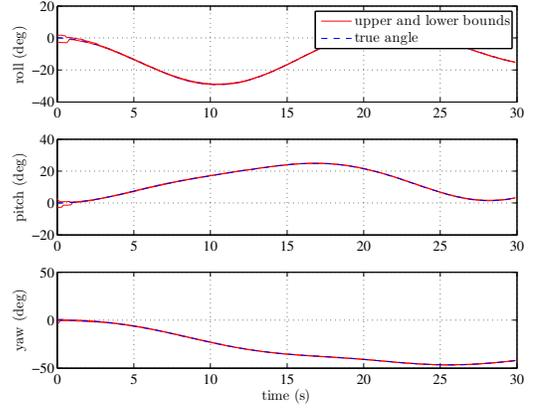
Fig. 1. Euler angles representation of the true state and the upper and lower bounds on the attitude estimates - simulation with noise-free angular velocity measurements.
