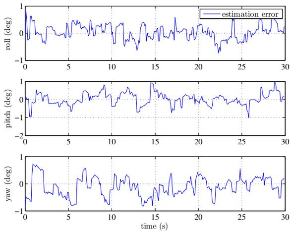
Fig. 4. Estimation error - simulation with noisy angular velocity measurements.
