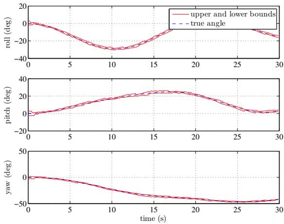
Fig. 3. Euler angles representation of the true state and the upper and lower bounds on the attitude estimates - simulation with noisy angular velocity measurements.
