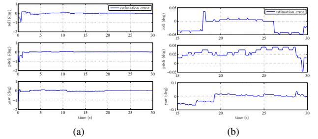
Fig. 2. Estimation error - simulation with noise-free angular velocity measurements.
