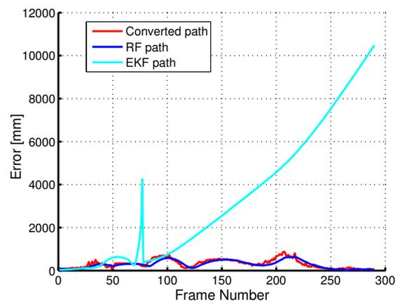
Fig. 4. Errors in RF and EKF
