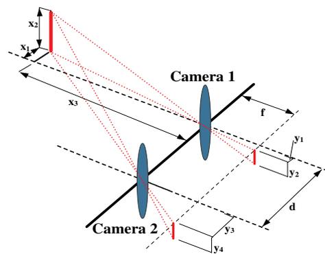
Fig. 1. The principle of perspective projection.
