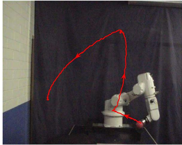
Fig. 2. End effector measured path from the video sequence
