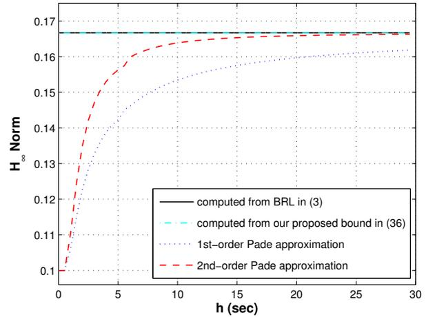
Fig. 1.  $H_\infty$  norm of the symmetric delayed system determined using different methods
