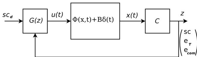
Fig. 5. State feedback control scheme for system model (3).
