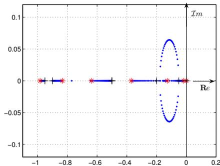
Fig. 2. The trajectories of the poles of  $A$  for increasing values  $\bar{e}_B$ . All the poles lie within  $\text{Re} \leq 0$ .
