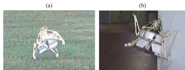
Fig. 1. The DFAV overturning during a take-off maneuver (a) and interacting with a wall (*set-stand*) (b).
