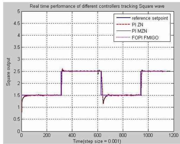
Fig. 16. Real-Time control of water level in cascaded control configuration.
