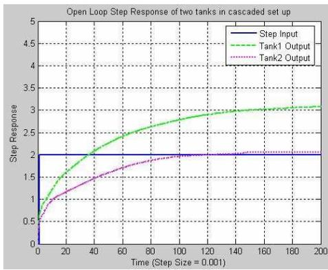
Fig. 14. Open loop step response of two cascaded tanks.
