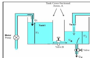
Fig. 13. System model for cascade control coupled tank.
