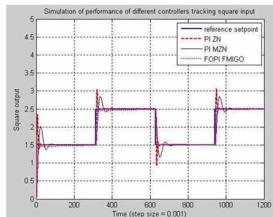
Fig. 6. Simulated control of water level in first order SISO configuration.
