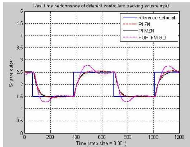
Fig. 12. Real-Time control of water level in second order SISO system configuration.
