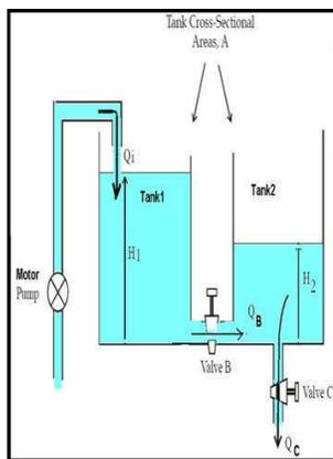
Fig. 8. System model for second order SISO coupled tank.
