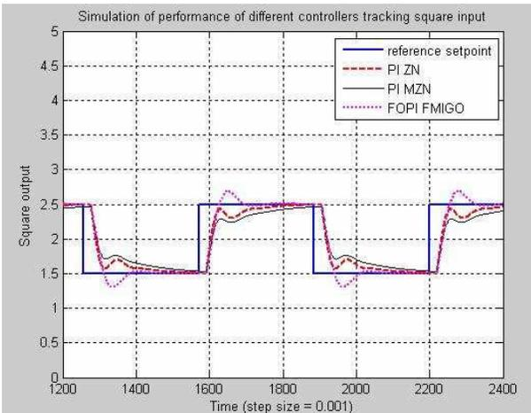
Fig. 11. Simulated control of water level in second order SISO system configuration.
