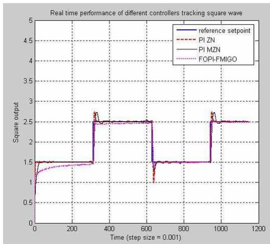
Fig. 7. Real-Time control of water level in Case-I configuration.
