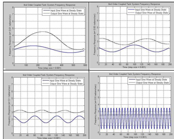
Fig. 9. Frequency response of second order SISO coupled tank system.
