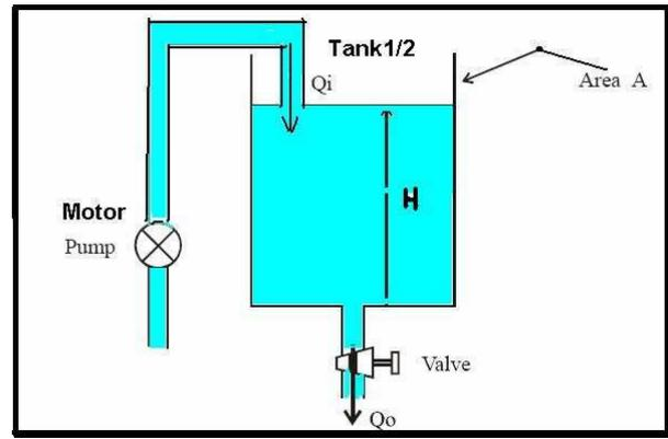
Fig. 3. System model for first order SISO coupled tank.
