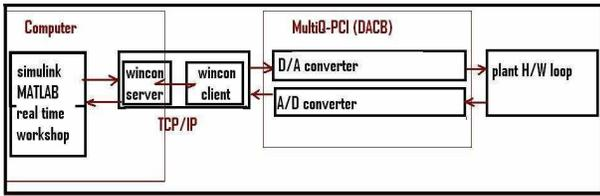
Fig. 2. Schematic of the real-time, hardware-in-loop experiment platform.
