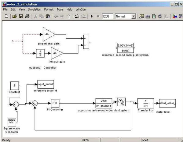
Fig. 10. Simulink block diagram of water level control in second order SISO system configuration.
