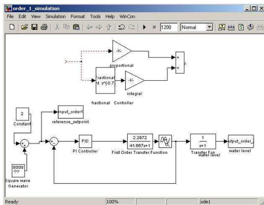
Fig. 5. Simulink block diagram of water level control in first order SISO configuration.
