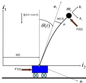
Fig. 2. A flexible inverted pendulum on a cart
