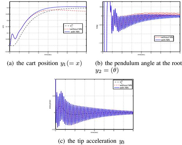
Fig. 4. Time responses with and without NN augmentation for the decentralized controllers
