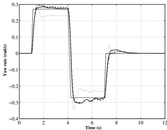
Fig. 4. 50° steer reversal test at 90 km/h. Thin line: reference yaw rate. Comparison between the yaw rate courses obtained with the uncontrolled vehicle (dotted) and with the controlled ones using either yaw rate sensor (solid) or DVS (dashed).
